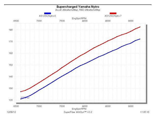
Here's a graph comparing stock boost F1100 turbo with stock tune and with the \$289 D&D reflash along with the Yamaha Nytro SC with 28/28 tooth pulleys and overdrive pulleys. Note that the overdriven Nytro supercharger, even with the fuel tuner maxed out, caused A/F ratio to lean out at high revs causing HP to tail off. More fuel is necessary to overdrive the SC.
