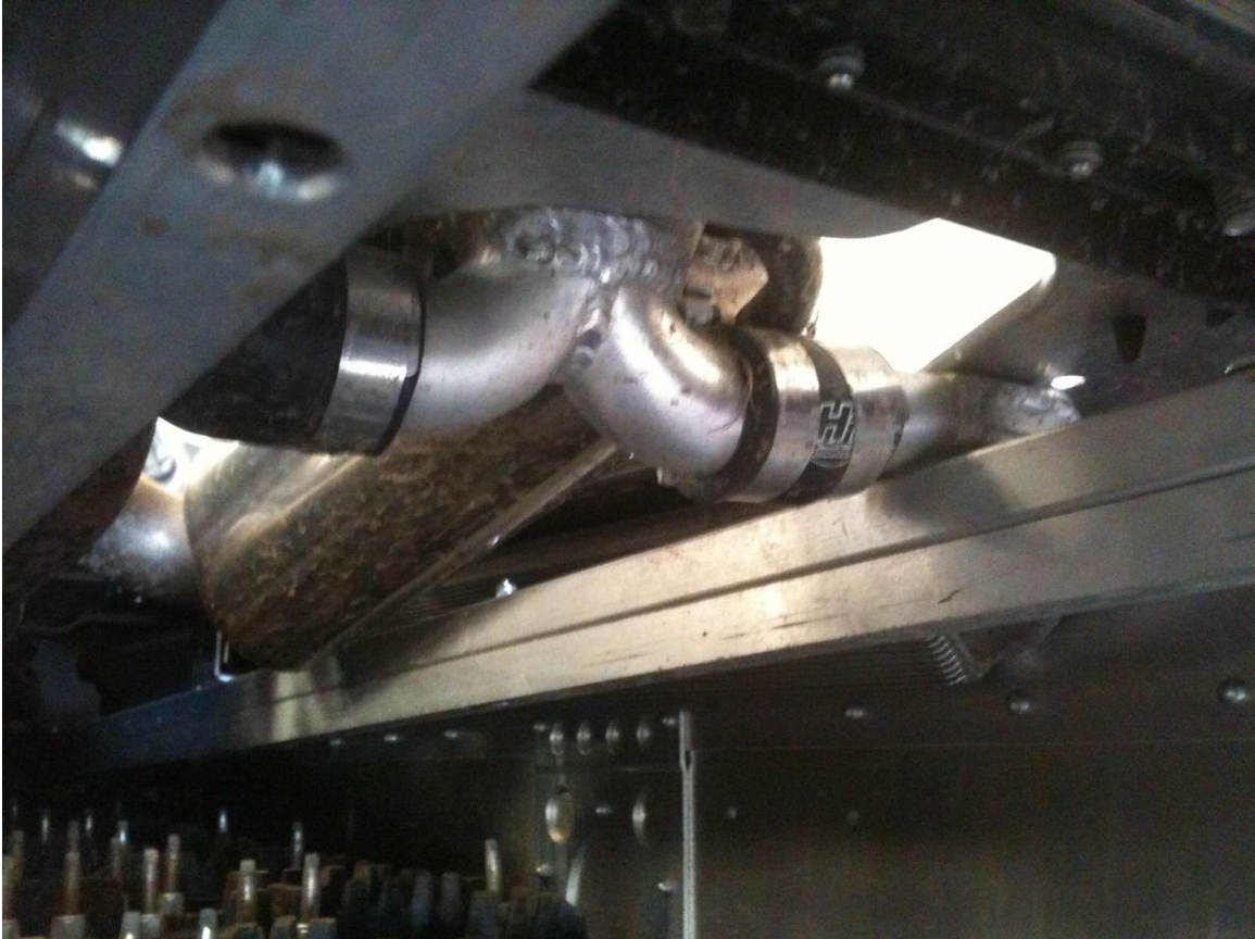
Here's a photo of the split turbo compressor outlet viewed from under the sled tunnel. The finned extrusions can be seen on the right side of the stock engine heat exchanger.
